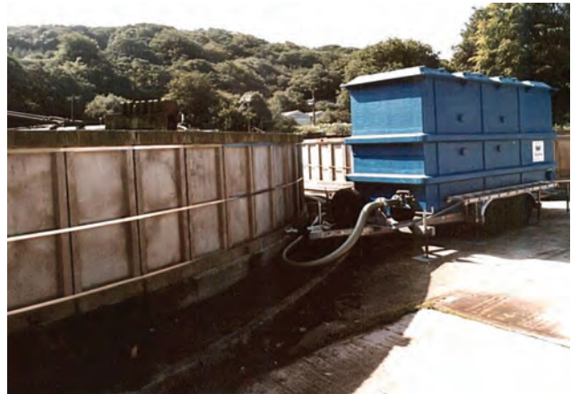
SAF units can be trailer-mounted for mobility, making them ideal for emergency, supplemental, or temporary use, or for pilot studies.
