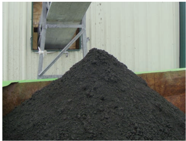
Solids generated by the Volute Dewatering Press.
